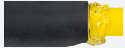
Photo 15: Close up of hot-melt adhesive fillet at sleeve end
