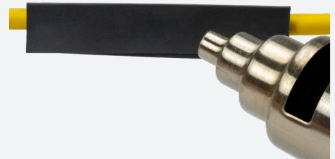
Photo 3: Nozzle focused near tubing center on overlap seam
