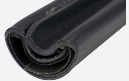
Photo 12: Overlap seams curled up prior to full shrinkage.
