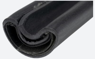
Photo 4: Overlap seams curled up prior to full shrinkage.
