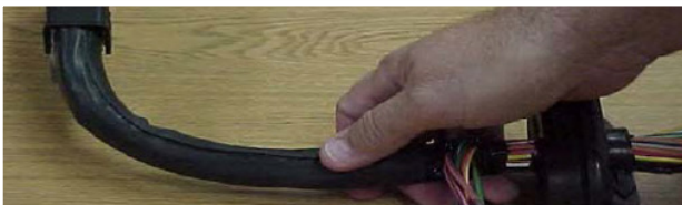
Photo 4: Rubbing adhesive seam after shrinking.
