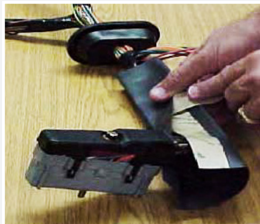
Photo 1: Installing PRT® around the cable
