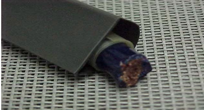
Photo 9: PRT aligned over Z-Block tape
