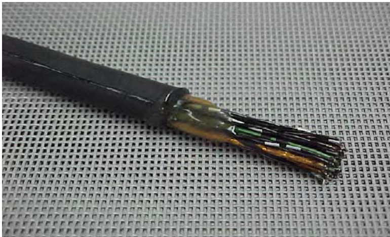
Photo 7: PRT fully shrunk around water blocked end
