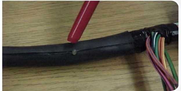
Photo 8: Residual adhesive ball
