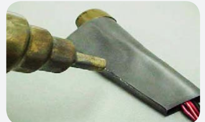
Photo 5: Shrinking tubing using a reducer nozzle.
