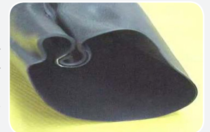
Photo 6: Overlap seams curled up prior to full shrinkage.
