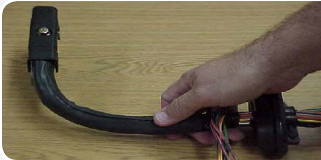
Photo 7: Rubbing adhesive seam after shrinking.
