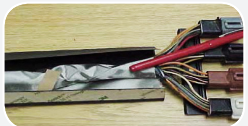
Photo 3: Shield layer wrapped around cable bundle
