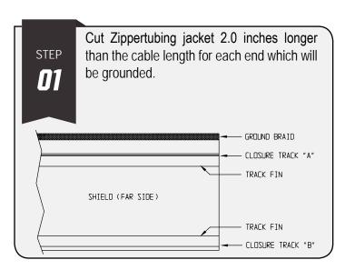
Pull the stitching from the braid back 2.0 inches from the end of the jacket and then cut off the loose braid. Cut the loose portion of track "A" and along the edge of the track "B" back 2.0 inches each.
